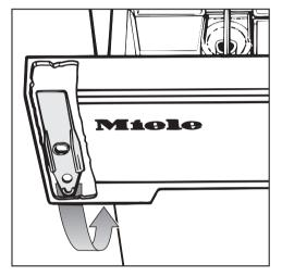
To clean the lint trap, remove the tool from behind the detergent dispenser drawer.
